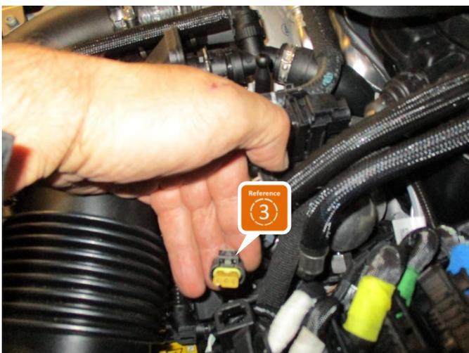
Connect the adapter cable in between camshaft sensor and sensor plug.
