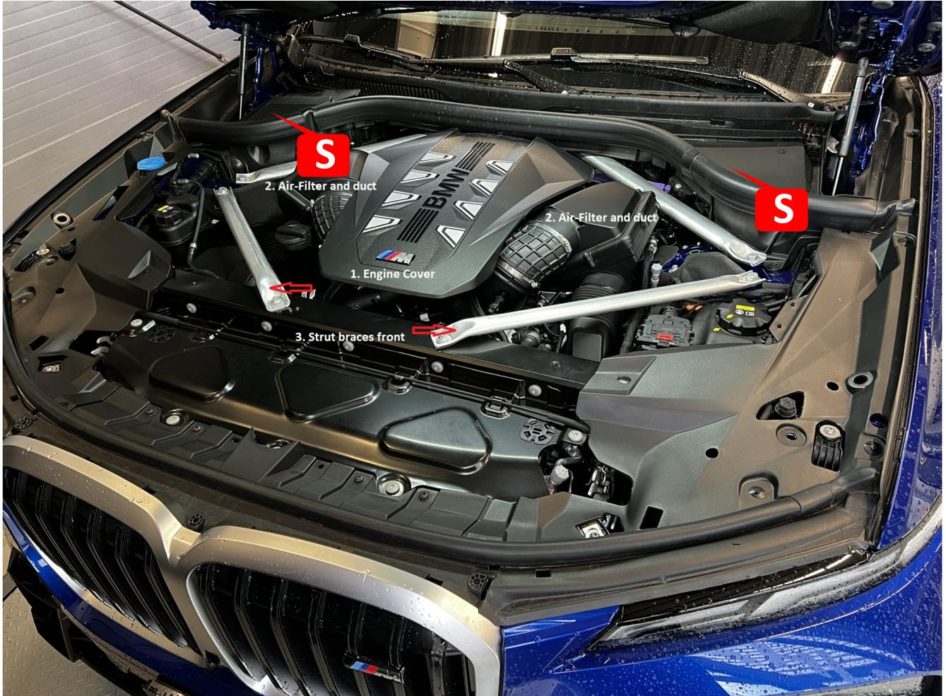
Numbers 1 - 3 are parts that need to be removed before installing the engine performance upgrade
