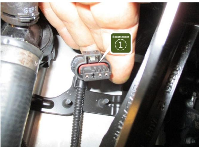
Disconnect the boost pressure sensor connector by unlocking the locking lever from the boost pressure sensor. Connect the adapter cable in between these connection.
