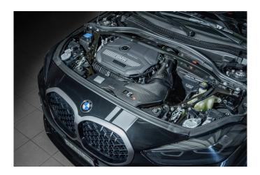
Open the engine hood. Remove the engine cover. The engine cover is not screwed.
