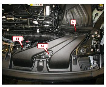
Localise the right area from the engine compartment. Solve the screws (S1) and (S2) and remove the air filter suction tube. Unlock holder (H) for removing it.
