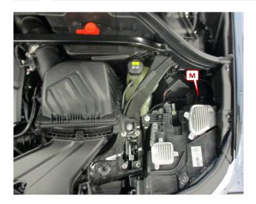
Move the adapter cable not in parallel with injection pipelines or ABS-control device connecting leads. Keep to very big distances. Fix the adapter cable with cable ties. Connect the module with the adapter cable. Check all connections again and reassemble the vehicle in reverse order.
