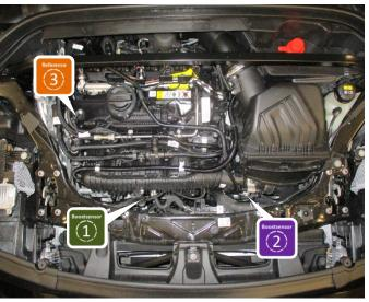
Connect the system to these three sensors. Intake manifold pressure sensor, boost pressure sensor and camshaft sensor. The 3-pin intake manifold pressure sensor is located in front of the intake manifold. The 4-pin boost pressure sensor is located in the front, right area at the intake pipe before throttle valve. The 3-pin camshaft sensor is located on the left side top of the engine.
