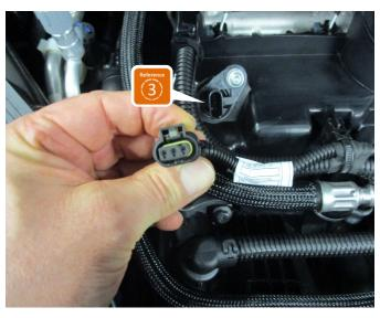
Open the plug by unlocking the locking lever. Connect the camshaft adapter in between both connections.
