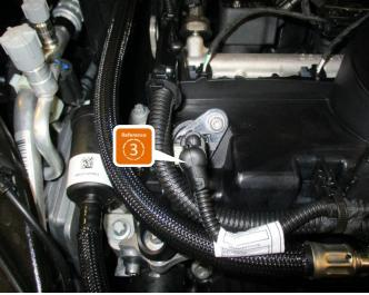
Localise the 3-pin camshaft pressure sensor on the left side, top of the engine.
