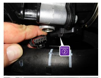
Open the plug by unlocking the locking lever. Connect the boost pressure adapter in between both connections.
