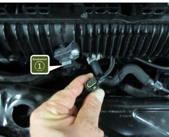
Open the plug by unlocking the locking lever. Connect the intake pressure adapter in between both connections
